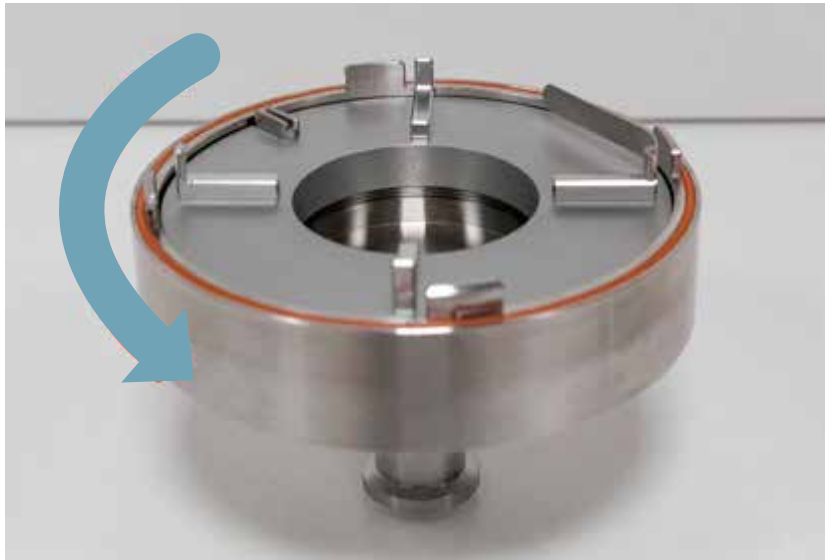
Figure 3-6. Rotate the plate holder counterclockwise to remove it
