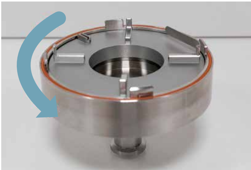
Figure 3-3. Rotate plate holder counterclockwise to increase its height
